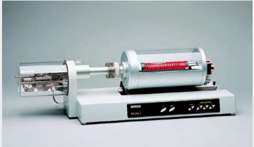
DIL 402 C/7 with 2000 °C furnace (cut-away view)
