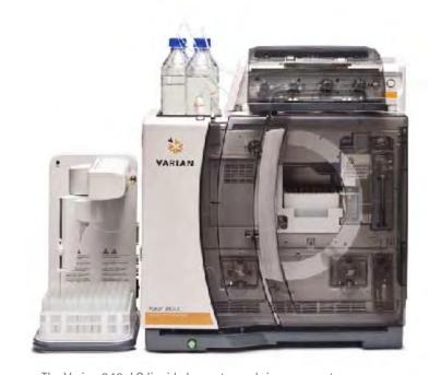
The Varian 940–LC liquid chromatograph is a compact, stylish, fully-integrated HPLC, delivering versatility, reliability and scalability.
