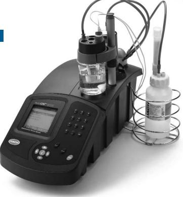
The world's first automated amperometric titrator dedicated to measurement of free and total chlorine, chlorine dioxide, chlorite, and sulfite. Built-in titration procedures are virtually free from error and uncertainty. The AutoCAT™ 9000 Titrator
