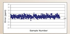
Exact mass measurement over long time periods. Compound X was analyzed via repeat injections over a time course of 10 days. The mean RMS mass measurement error for these data = 1.9 ppm.
