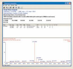
With exact mass measurement (sub 5 ppm) and isotope interpretation with MassLynx Software (i-FIT), there are only two possible elemental compositions with the top results being the correct formula.
