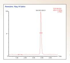
This example shows 10 pg of reserpine injected oncolumn. S/N is typically in excess of 100:1.
