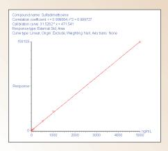
This example of sulfadimethoxine (0.5-5000 ng/mL) demonstrates up to 4 orders linear dynamic range with DRE enabled.
