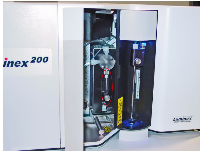
Frontal view of a Luminex system with door open and syringe exposed.
