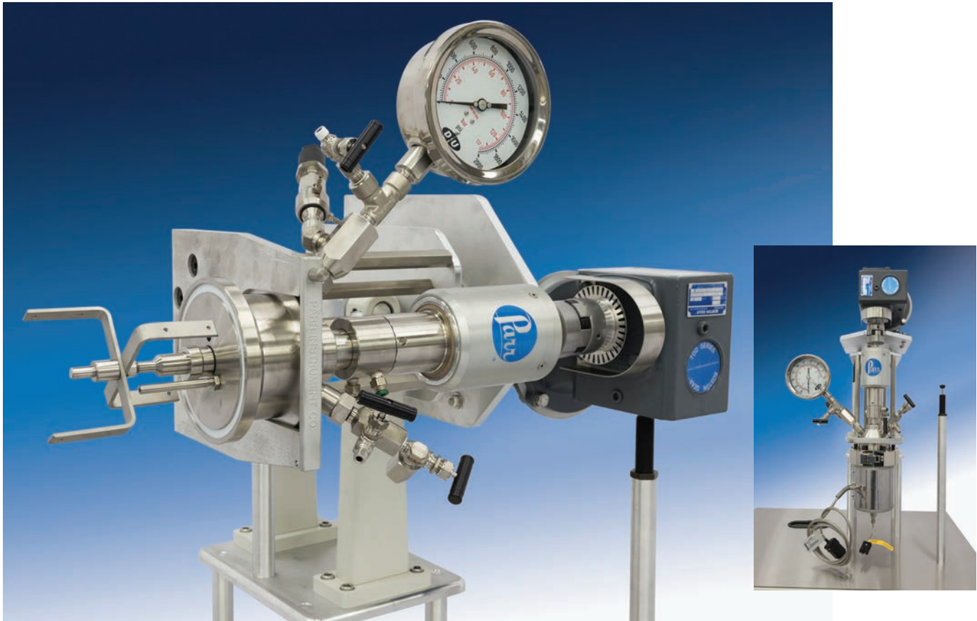
This one liter reactor can be oriented vertically for loading or tilted horizontally for stirring. A heavy-duty stirring motor and double anchor stirrers are used. Another option would be to tilt upside down for discharge. An optional flexible mantle heater (not pictured) can be used to obtain temperatures up to 350 C. Maximum pressure is 1900 psig for this system.
