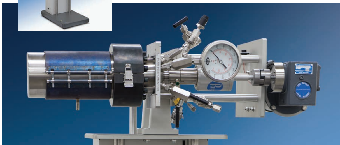
The 4578 Pressure Reaction System shown above is a 1.8 L, fixed head reactor is mounted on a floor stand and is rated for temperatures up to 500 °C with a maximum pressure of 5000 psig. In the horizontal position, the internal stirrers tumble the material rather than try to stir it with a standard vertical stirrer. These custom reactors are secured vertically for loading and then safely tilted horizontally for stirring.
