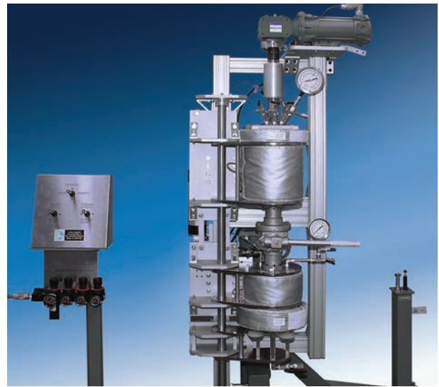
The reactor shown in the two images above and right has a five gallon capacity, and is used for stirring horizontally. Pneumatic controls on the left can tilt the system upright to open the bottom drain valve. The product is filtered and collected in the lower heated sample collection vessel. This system is used for producing synthetic fabric from biomass as an alternative to a petroleum-based process.
