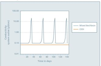
When a mixed bed ion exchange cartridge is used, the conductivity of the product water increases during normal operation and exhaustion. Cartridges have to be changed if the maximum acceptable conductivity is reached.
