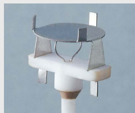
Sample carrier with Platinel® thermocouple
