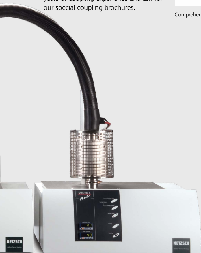
Coupling of Tensor 27, external gas cell, TG 209 F1 Libra™ and QMS 403 C Aëolos®
