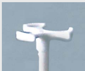
Standard Al 2 O 3 sample carrier for corrosive gases
