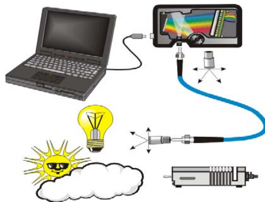
Figure 6-4: Typical Relative Irradiance Setup. A light source with a known color temperature (such as the LS-1 or LS-1-LL - lower right) is used to take a reference spectrum. The light to measure (lower left) is accumulated through a CC-3 Cosine Corrector (or FOIS integrating sphere) into an input fiber, which carries the light information to the spectrometer. The spectrometer then transmits the information to the PC, which compares the measured spectra against the reference spectrum, thus removing wavelength-dependent instrument response from the measurement.
