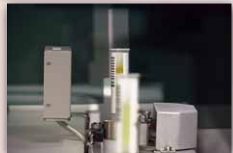
'Point-in-space' pipetting technology, used when connected to automation systems, helps prevent bottlenecks in sample processing.
