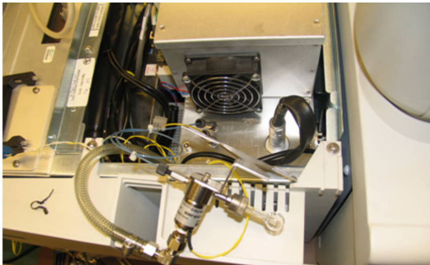
Figure 24 Removing the reference gas vial from the mass spectrometer
