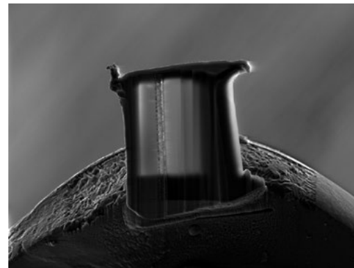
Ultra-thin TEM lamella showing interface zone on Si. Transparent area is homogeneously thin.
