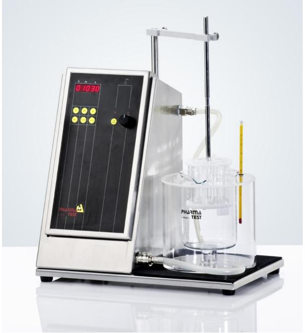
The PTZ-S is a manual tablet disintegration testing instrument, manufactured according to the recent USP <701/2040>, EP <2.9.1/2.9.1.2>, JP and other pharmacopoeias.
