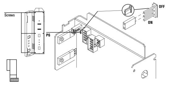
Figure 26. P6 jumper setting
