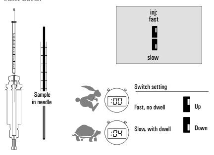
Figure 54. Switches for setting the injection speed
