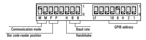
Figure 14. Setting the address switches
