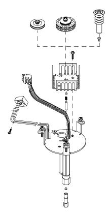
Figure 76. Inlet assembly
