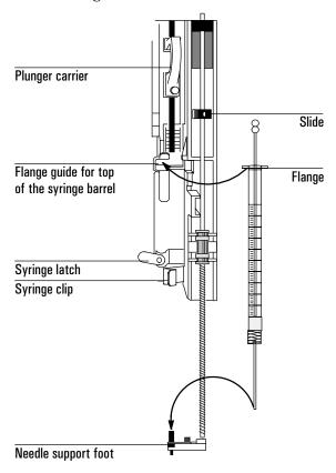
Figure 84. Installing the syringe for 250- or 320- $\mu$ m on-column injection
