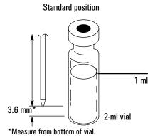
Figure 43. Variable sampling depth
