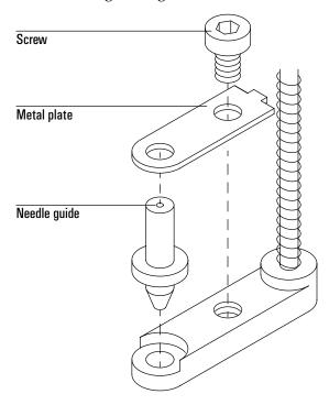
Figure 85. Needle support foot for 250- $\mu$ m injection
