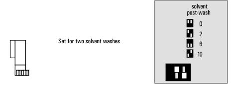
Figure 58. Switches for setting the number of solvent washes
