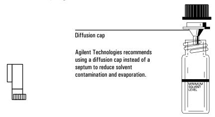
Figure 27. 4-ml bottle used for solvent and waste
