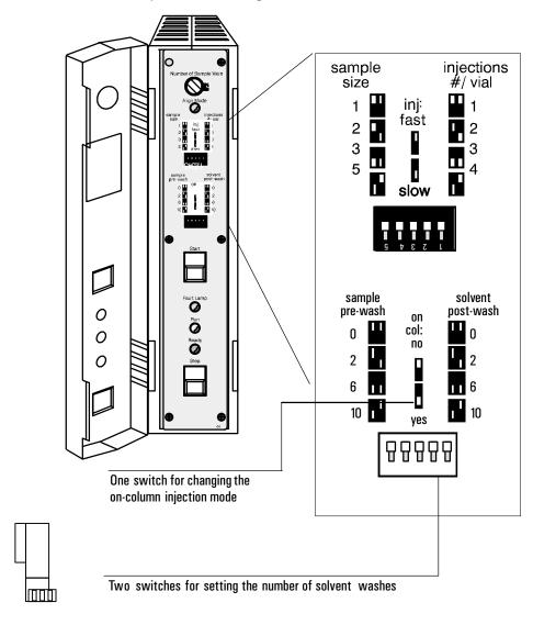
Figure 52. Switches for setting six injector parameters
