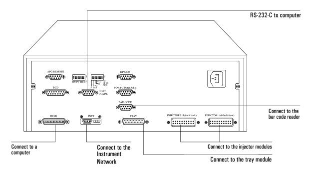
Figure 13. Common cable connections
