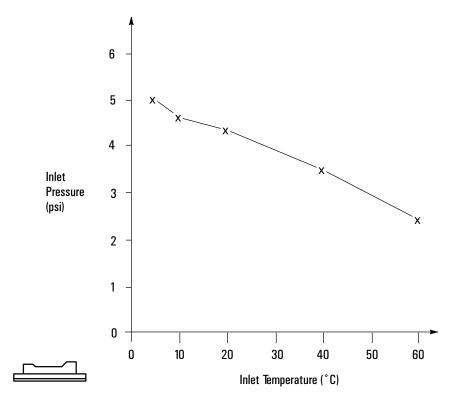
Figure 89. Maximum inlet pressures and temperatures
