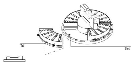
Figure 11. Inserting the tray quadrants
