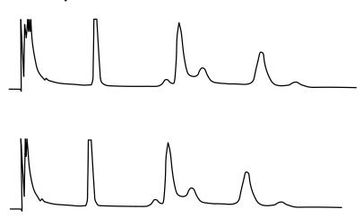
Figure 68. Retention times or areas are not reproducible
