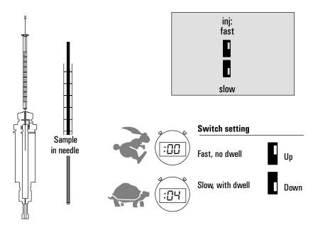
Figure 42. Injection speed
