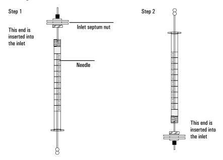
Figure 77. Ensuring proper alignment
