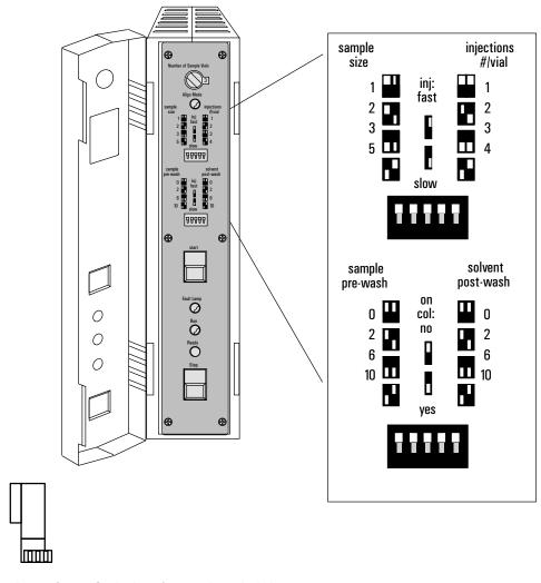
Figure 64. Switches for setting six injector parameters
