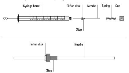
Figure 73. Syringe parts and assembly
