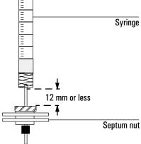
Figure 79. Verifying column installation
