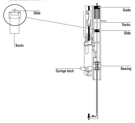
Figure 82. Cross-section of slide alignment
