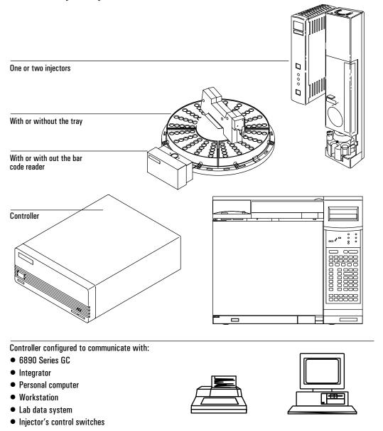
Figure 1. The automatic liquid sampler as part of your analytical system
