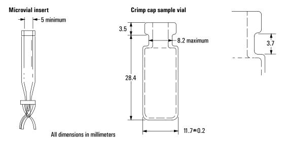
Figure 18. Dimensions for sample vials and microvial inserts
