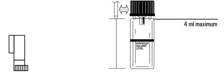
Figure 29. Shows position of syringe tip when dispensing waste
