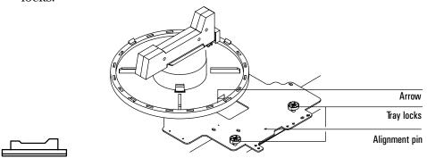
Figure 9. Attaching the tray
