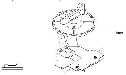
Figure 8. Threading the tray cable
