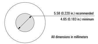
Figure 19. Specifications of vial cap aperture
