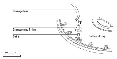
Figure 86. Attaching the tray drainage tube fitting
