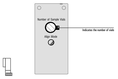
Figure 60. Setting the rotary switch for three sample vials
