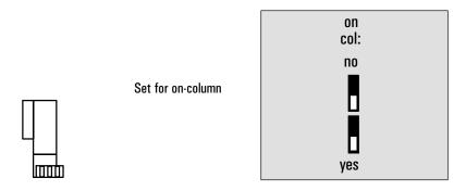
Figure 57. Switch for setting the on-column injection mode
