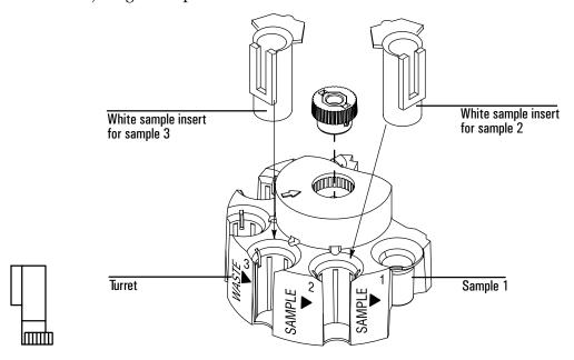
Figure 66. Placing sample inserts for three sample vials
