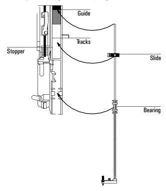
Figure 81. Installing the 250/320- $\mu$ m needle support assembly
