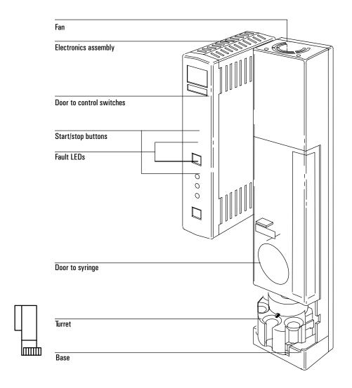
Figure 3. G1513A injector module
