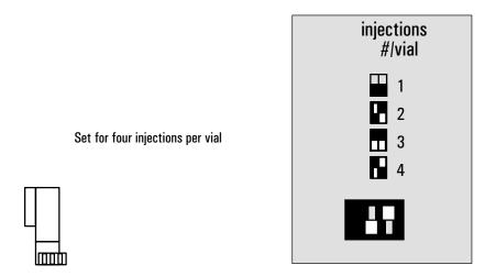
Figure 55. Switches for setting the number of injections from each sample vial
