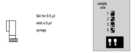
Figure 53. Switches for setting the sample size
