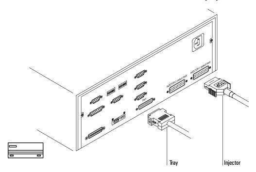
Figure 16. Connecting the injector and tray cables
