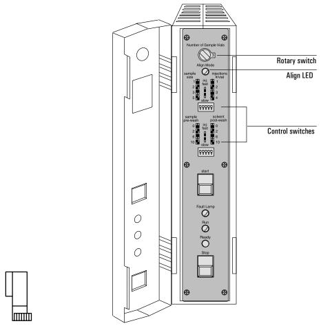
Figure 4. The parameter control switches
