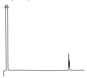
Figure 71. Blank run showing carryover peaks
