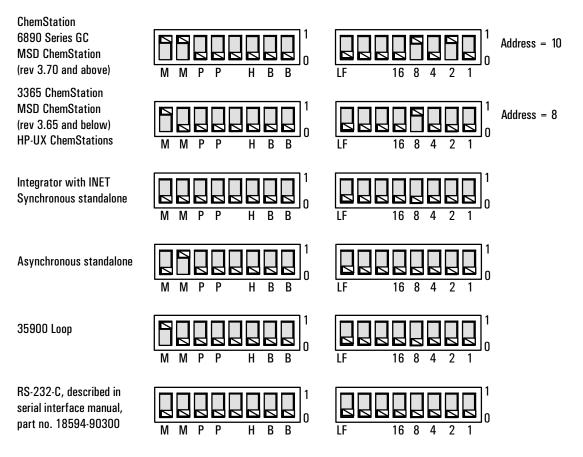
Figure 15. Examples of switch settings
