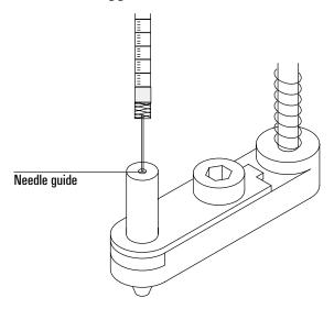
Figure 83. Needle support for 250- $\mu$ m injection
