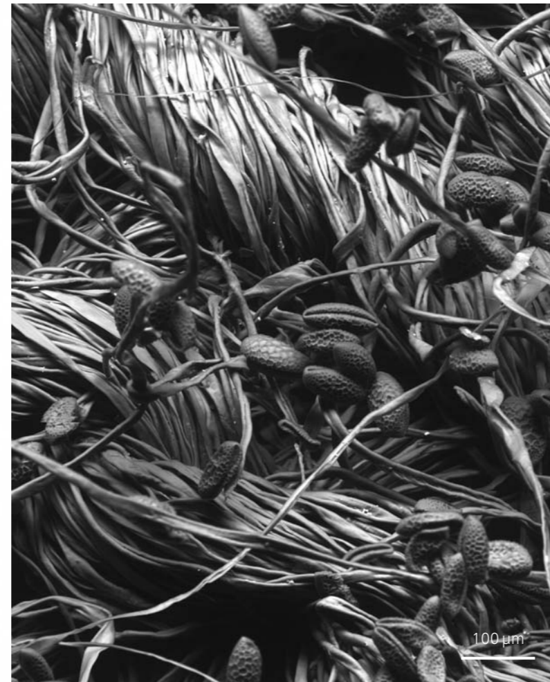
Pollen on fabric imaged in water vapour at 20 kV using the BSE detector.
