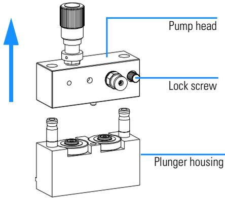
**4** Remove the support rings from the plunger housing and lift the housing away from the plungers.
