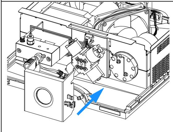
**10** Replace the top foam section, optional interface board (if installed), metal cover and top cover (see “Replacing the Top Cover and Foam” on page 156). Replace the pump on stack, reconnect all tubings and cables.
