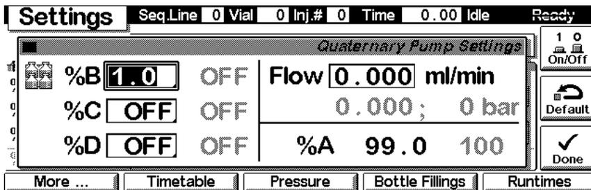
Use the **m**-key for the context sensitive menu. The **Status** command pulls up a monitor screen displaying signals and spectra as programmed. **Reset** will load the pump default parameters.
