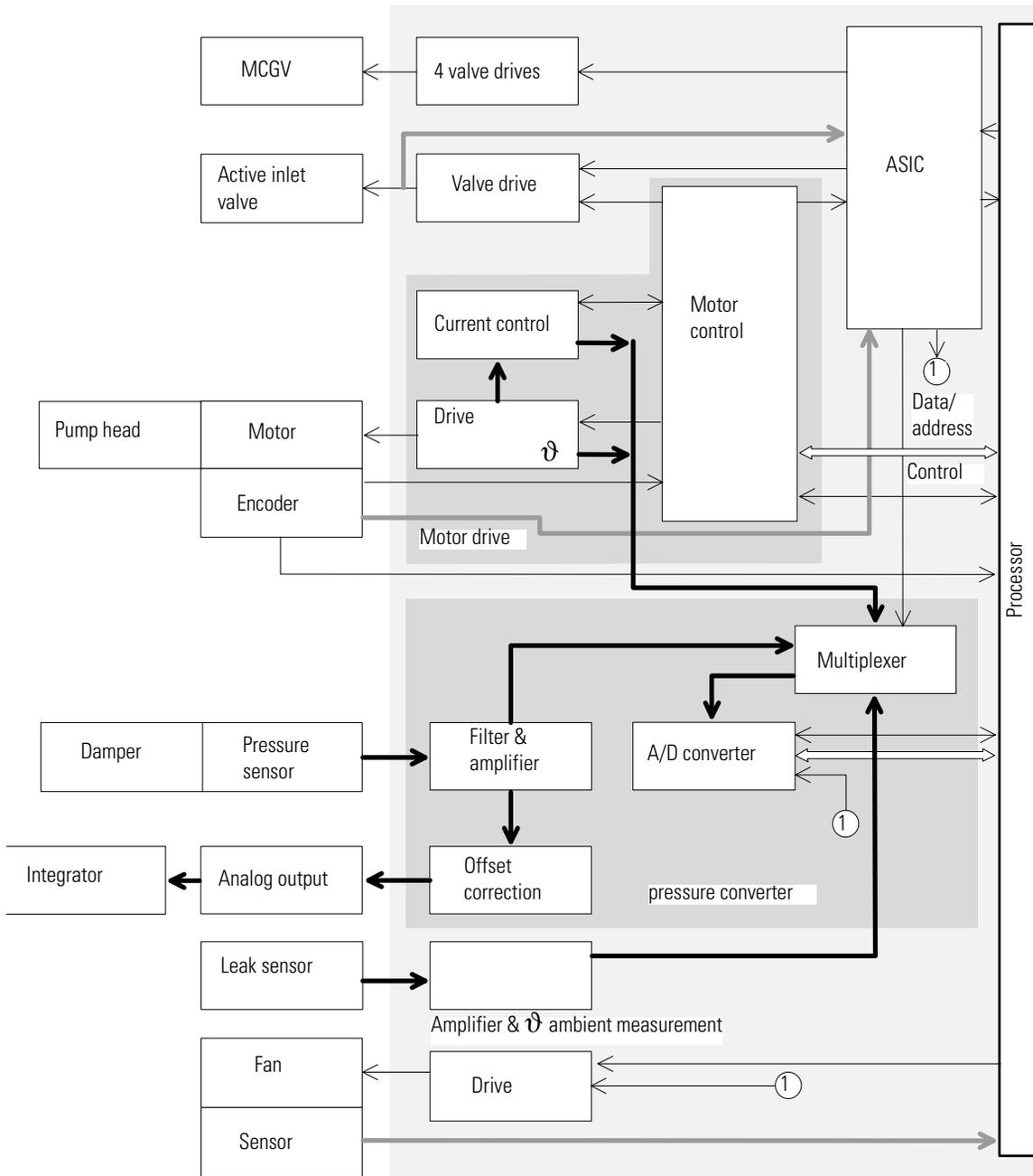
The Low-Pressure Pump Main Board (LPM)
