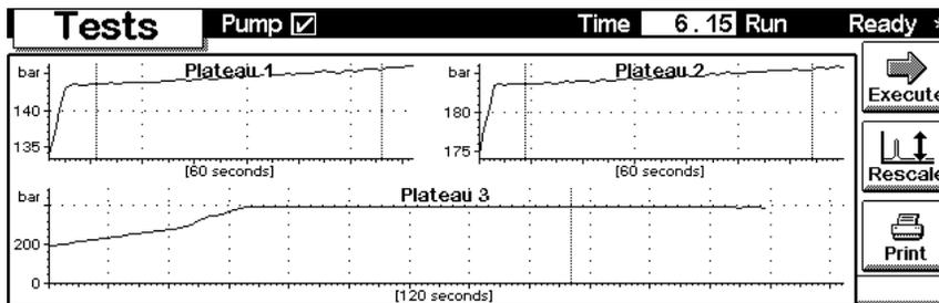
**Diagnostics and Tests****Pressure Test**
