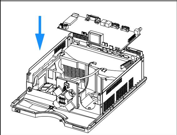
**14** Re-install pump assembly, fan and damper into the bottom foam and re-connect to the main board.
