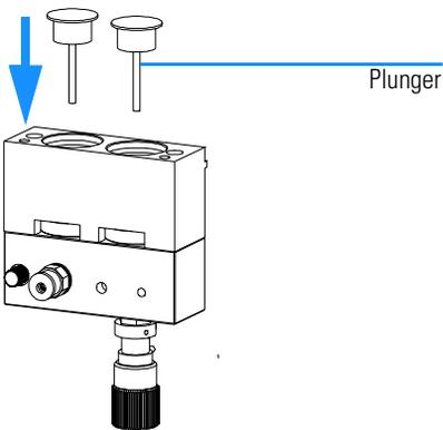
**3** Tighten the lock screw.
