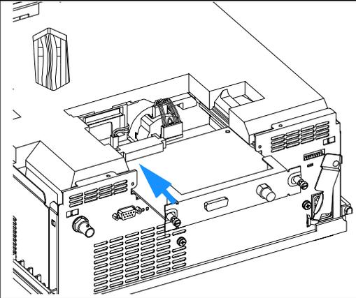
**5** Replace the metal cover (slide the metal tabs into place (1) underneath the Z-Panel in the front, then lower the back of the metal plate (2)) and fix the two holding screws.
