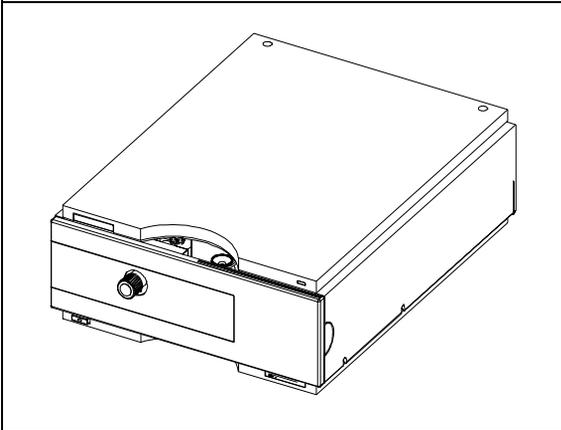
**2** Remove the gradient valve (MCGV) cover (see “Exchanging the Multi-Channel Gradient Valve (MCGV)” on page 123).
