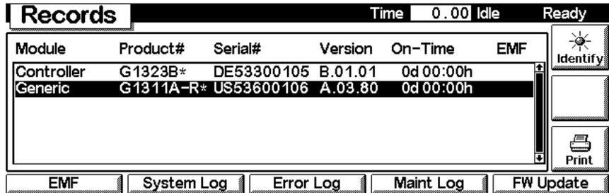
Use the F5 key (**FW Update**) to enter the Update section. Select the a file from the PCMCIA card (1311nnnn.DLB) and press execute. When the update has finished, press F7 key (**Transfer**) to return the module into the normal mode (LED on module should stay yellow).
