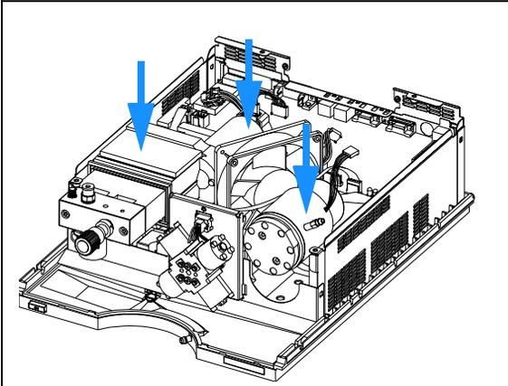
**15** Place the Z-panel into its position and tighten the two screws.
