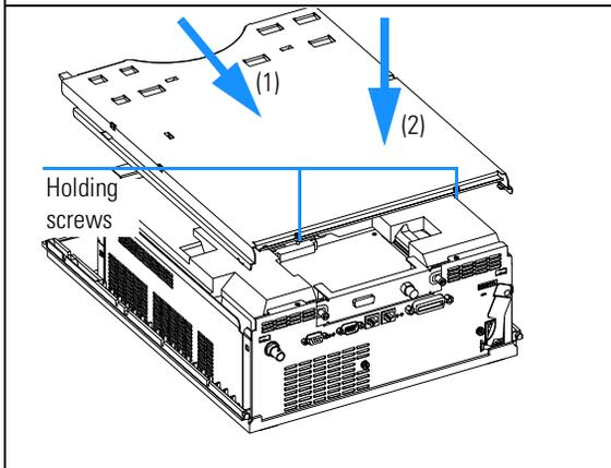
**6** Replace the top cover. Replace the pump on stack, reconnect all tubings and cables.
