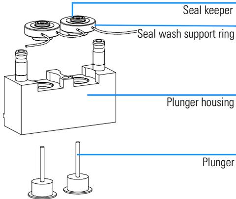
**7** If necessary replace the pump seals (see page 112 ). Reassemble the pump head (see page 121 ).
