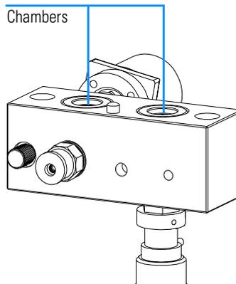
**4** Insert new seals into the pump head.
