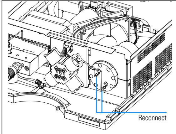
**9** Clip the valve cover into its position and connect the tubings back to the valve ports.
