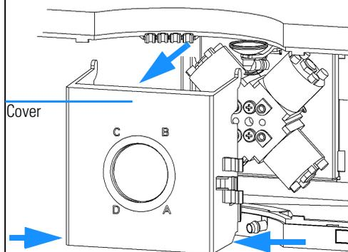
**3** Disconnect the MCGV cable, unscrew the two holding screws and remove the valve.
