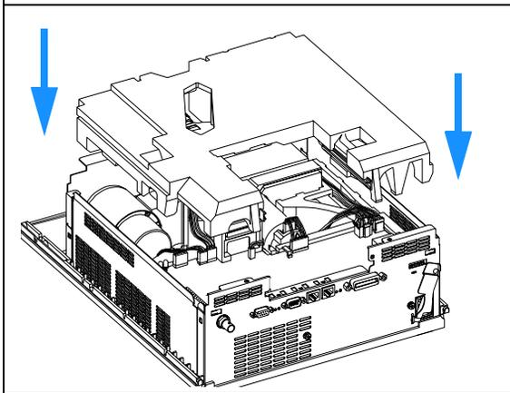
**2** Make sure that the foam is installed correctly and is located in the safety light switch.
