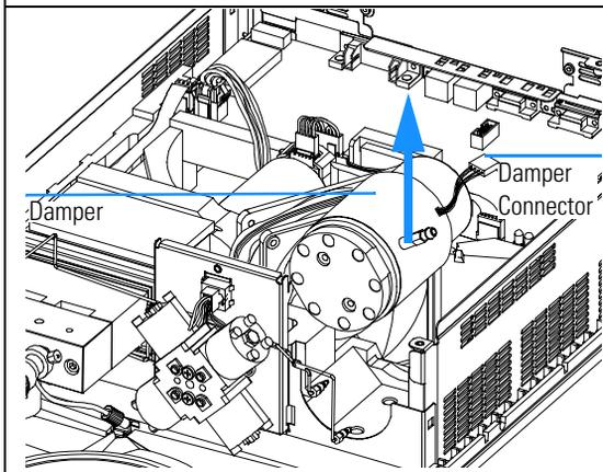
**6** Place the new damper into the recess and connect to the main board (J24).
