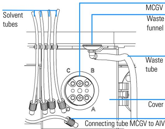
**2** Press the lower sides of the cover to unclip it. Remove the cover.
