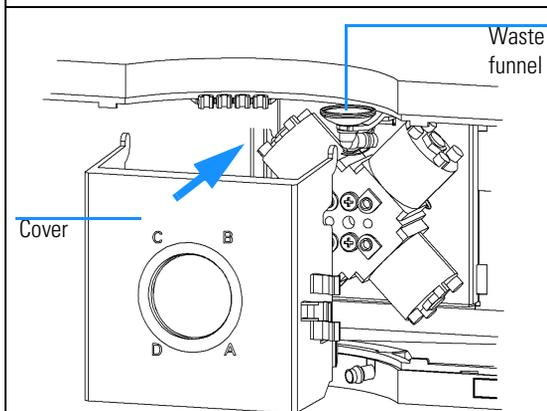
**6** Reconnect the tube from the active inlet valve to the middle position of the MCGV and then the solvent tubes at channel A to D of the MCGV. Make sure the orientation of the channels on the cover is labeled as shown below, otherwise re-label the cover.
