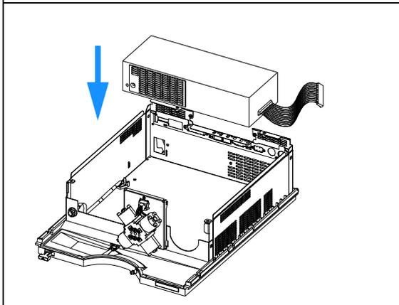
**11** Install the coupler onto the power supply switch and clip the light pipe back onto the coupler.
