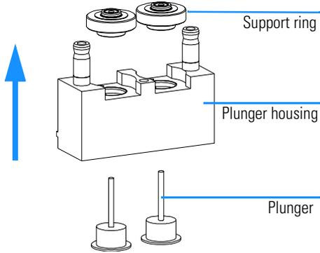
**5** Check the plunger surface and remove any deposits or layers. Cleaning can be done with alcohol or tooth paste. Replace plunger if scratched.
