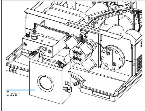
**3** Disconnect all capillaries and tubes from the pump head and disconnect the active inlet valve connector.
