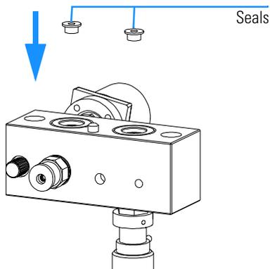
**5** Reassemble the pump head assembly (see “Reassembling the Pump Head Assembly” on page 121). Reset seal wear counter and liquimeter as described in the documentation.
