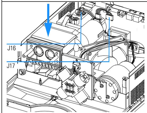
**8** Reinstall the pump head and fix with the two screws.
