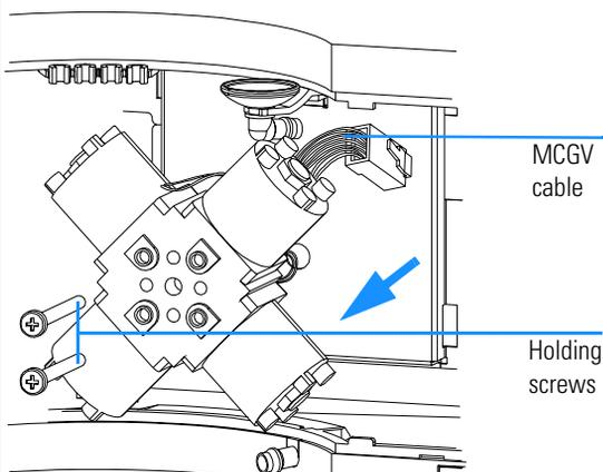
**4** Place the new MCGV into position. Make sure that the valve is positioned with the A-channel at the bottom-right position. Tighten the two holding screws and connect the cable to its connector.
