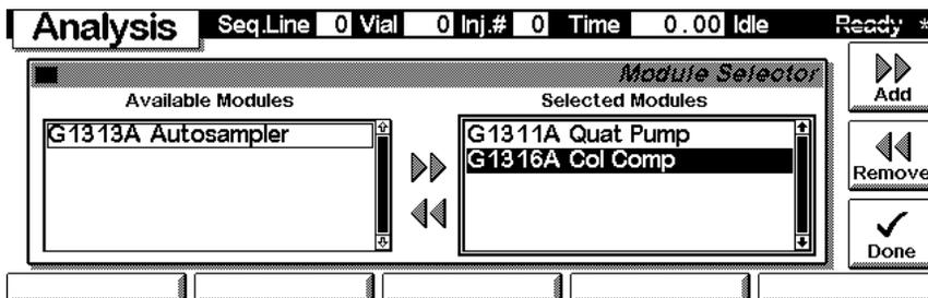
Here, e.g. the autosampler and thermostatted column compartment parameters are shown on the display as well. The number of parameters on the display is restricted as additional modules are added. A maximum of 4 modules is shown automatically. If more modules are connected to the system, you have to choose 4 of them in Setup view.
