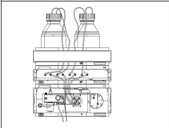
**9** Replace the leak funnel with the waste tube. Locate the lower end of the waste tube in the holder of the leak pan and clip tube to the holder at the gradient valve cover.
