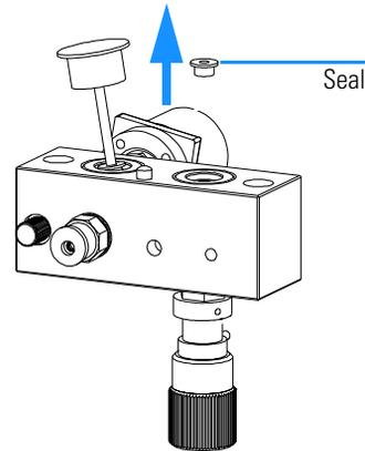
**Installing the Continuous Seal Wash Option**
