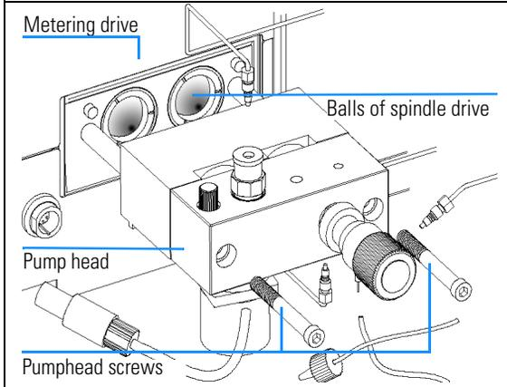
**5** Reconnect all capillaries, tubes and the active inlet valve cable to its connector.
