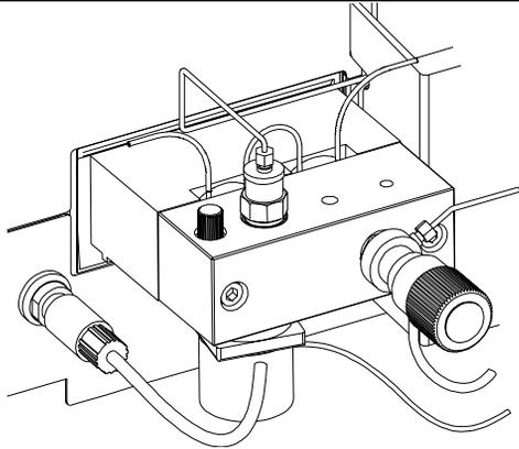
**2** Remove the seal keeper and the seal wash support rings from the plunger housing. Remove the seal keeper from the support ring assembly.
