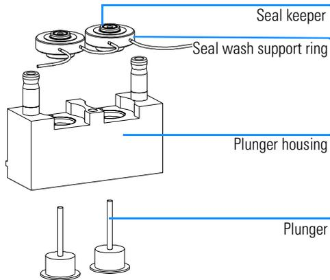
**3** Using the blade of a flat-blade screwdriver remove the seal wash gasket and the secondary seal from the support ring.
