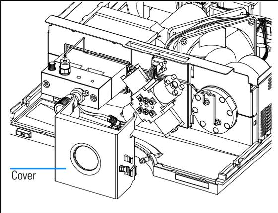
**11** Replace the pump on stack, reconnect all tubings and cables.
