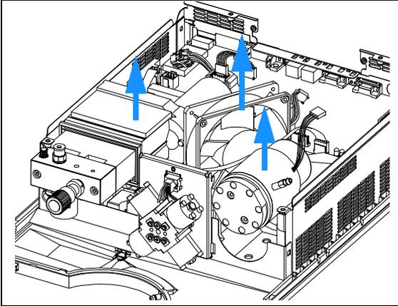
**5** Remove the LPM board, see “Exchanging the Low Pressure Pump Main Board (LPM Board)” on page 131.
