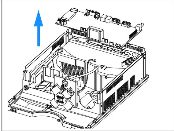
**6** Push the leak sensor cable through the recess in the foam and lift the bottom foam out of the instrument.
