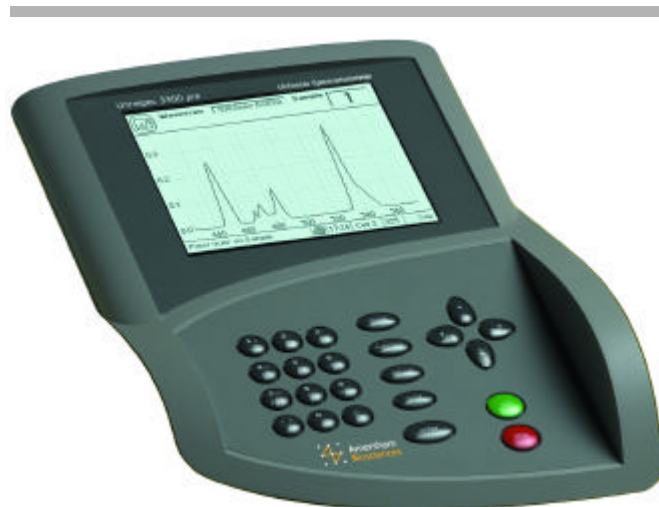
Figure 4. Ultrospec 3300 pro keypad and display
