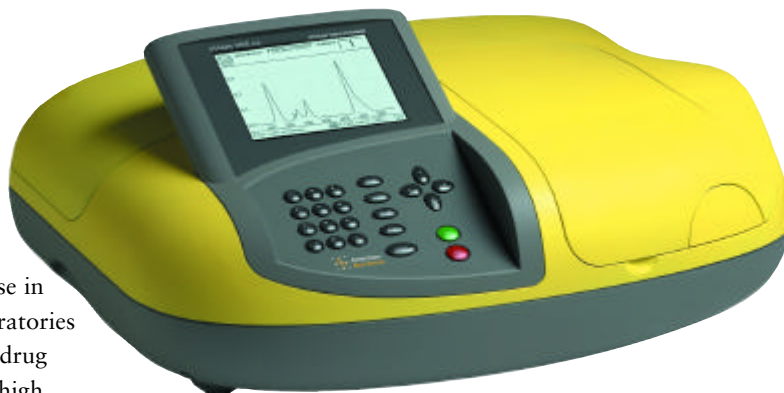
Figure 1. Ultrospec 3300 pro is a Pharmacopoeia compliant, stand-alone instrument with a high-resolution graphics display.
