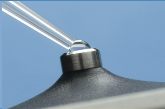
Pipetting 1 \mu l onto pedestal
