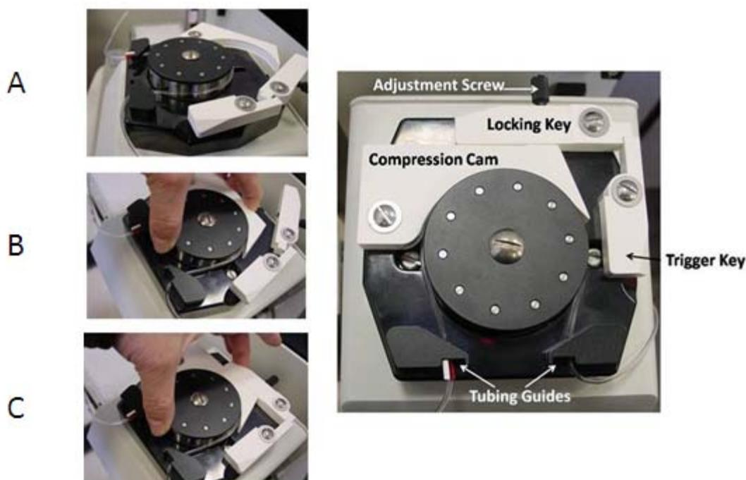
**Figure 2-7. Adjusting the peristaltic pump to optimize air gaps.**
