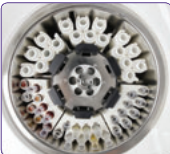
Combined sample and reagent disk for max 6 racks.
