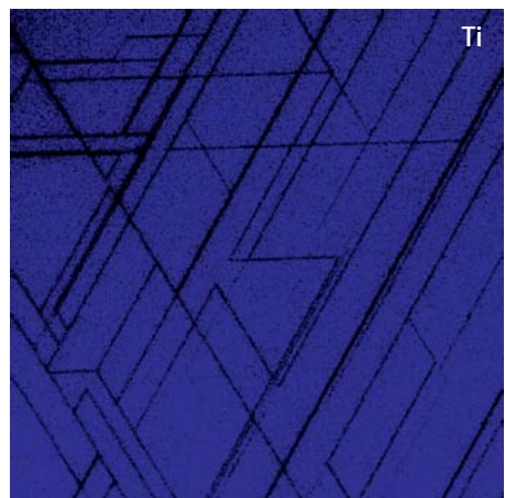
Figure 13: ChemiSTEM maps on WB/ \text{TiB}_2 / \text{CrB}_2 compound. HAADF image with chemical map of chromium, tungsten and titanium. All images are acquired simultaneously. Map size is 512 x 512 pixels acquired with 50 \mu\text{s} dwell time/pixel, 20 min total mapping time, and 1 nm spot size. Structures as small as 0.8 nm are visible in the chemical maps.
