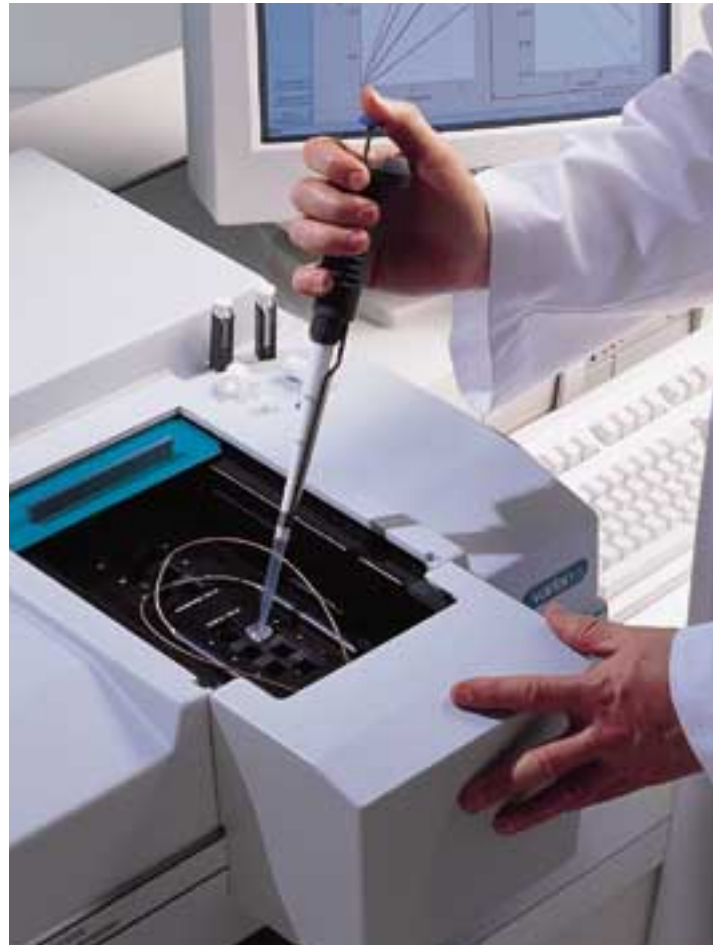
The Temperature Probe accessory allows the measurement of the temperature inside the cuvette.
